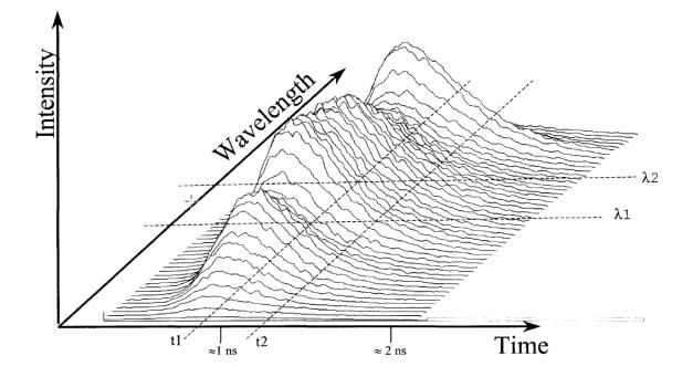
Ex. 1011, Fig. 3b. Figure 3b "illustrates how the time-resolved spectroscopy according to the invention results in an intensity 20 measurement as a
