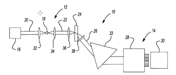
Ex. 1001, Fig. 1. Figure 1 shows laser source 16, high intensity light pulse 20 directed at nonlinear material member 18 (which can modify the optical
