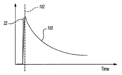
Figure 3 illustrates white light pulse 22, fluorescence 100, and delay line 102. Ex. 1001, 4:28–31, 5:30–33.
