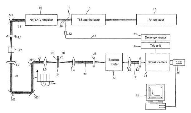
Ex. 1011, Fig. 1a. Figure 1a shows an Argon ion laser 12, "pumping" aTi:Sapphire laser 10, where the beam passes through amplifier 16, lenses L1,L2, and L3, to sample 24, before the beam is captured in streak camera 34.Ex. 1011, 6:26–7:23.
